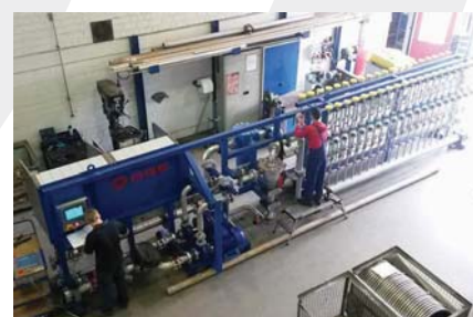
Final test of HTQ valve rack at Badische workshop prior to shipping
