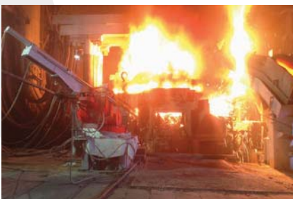
MultiROB with classic TempSamp function installed at NISCO (China) ...
